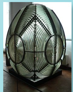
First-order rotating catadioptric Fresnel lens, dated 1870, displayed at the Musée national de la Marine, Paris. In this case the dioptric prisms (inside the bronze rings) and catadioptric prisms (outside) are arranged to concentrate the light from the central lamp into four revolving beams, seen by sailors as four flashes per revolution. The assembly stands 2.54 metres tall and weighs about 1.5 tonnes.
