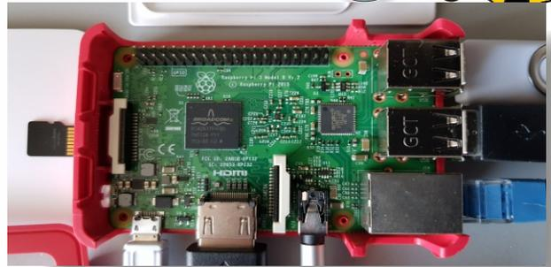
Figure 4 Raspberry Pi version 3 Model B V1.2 2015
