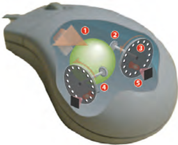
Figure 62: The internals of a mechanical mouse
