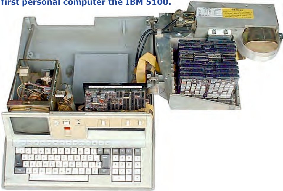
Figure 44: The Model 5100, IBM's first non-mainframe computer, believed to be the world's first portable computer.
