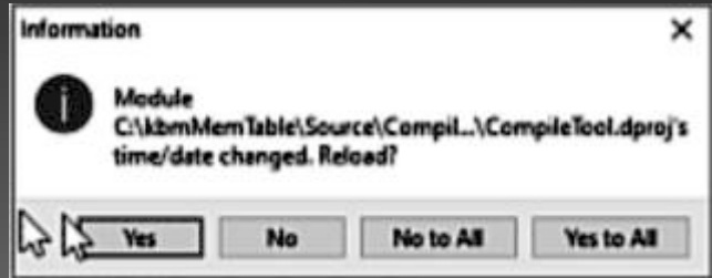
Figure 14: If you had compiled the program while Delphi was still running you can get this warning
