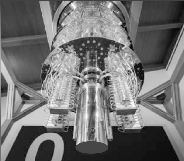
Figure 3: An IBM quantum computer where you can see the processor placed in the container at the bottom. Stephen Shankland/CNET
